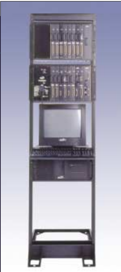
The Millennium 8-slot cabinets rack mounted with an eVPS Series 5000.
